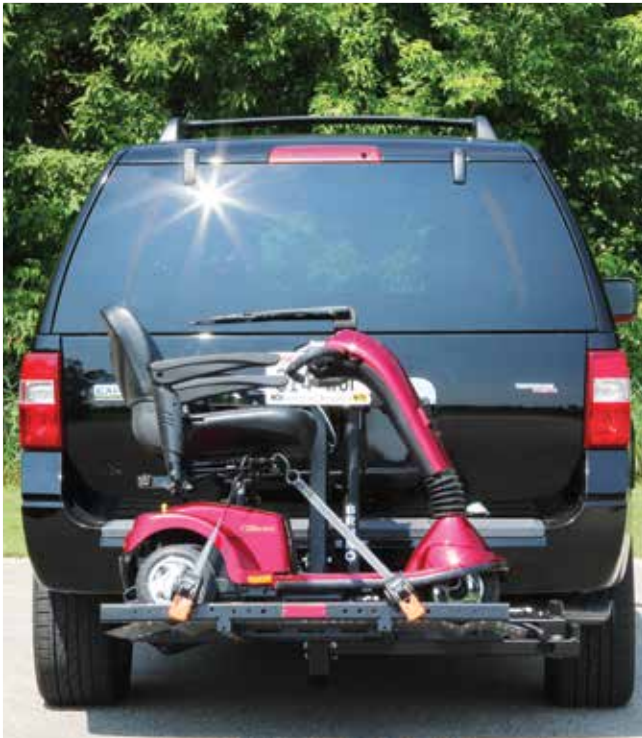
Hold-Tite foot securement for scooters (ASL-250A).
